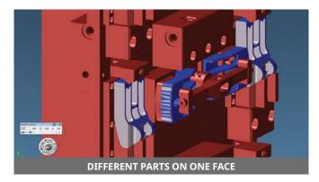
• The ability to generate CNC code in single-part mode to prove set up and machining before running a fully loaded tombstone
